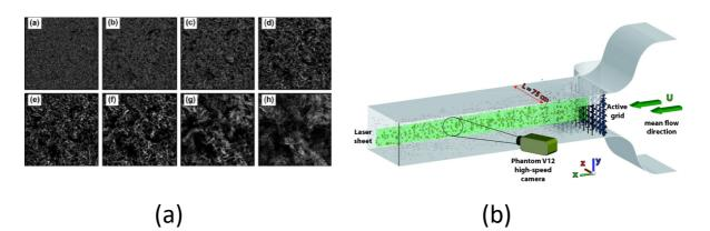
Figure 1: Illustration of the formation of clusters and voids from the simulations of Yoshimoto and Goto 2007 (a) and schema of the experimental set-up at LEGI (b).
